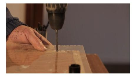
The hole I'm drill at the top of the box, is for the thermostat probe which will measure the temperature inside the tank and stop the thermostat from boiling further the oil.
