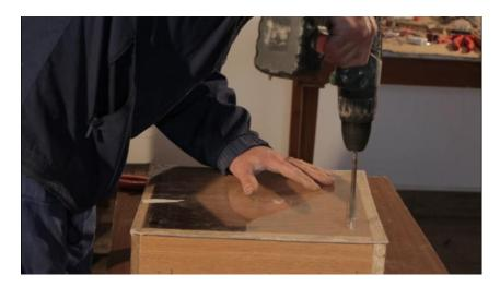
The other holes I drill are for the thermostat, which will set the boiling temperature.
