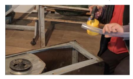
I am welding the tap with a short and long PVC pipe which will connect to the hose. For welding, you will need a PVC welding tool.
