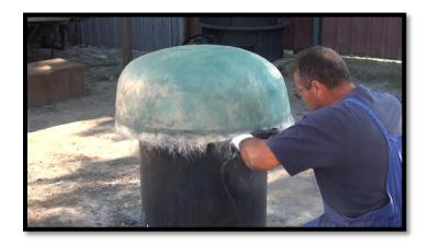
Now I start working on getting the finished dome out of it's mold.
