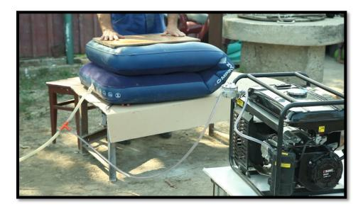
We start the generator on gasoline then we shut the gas and you can hear and see it running at 230 V.
