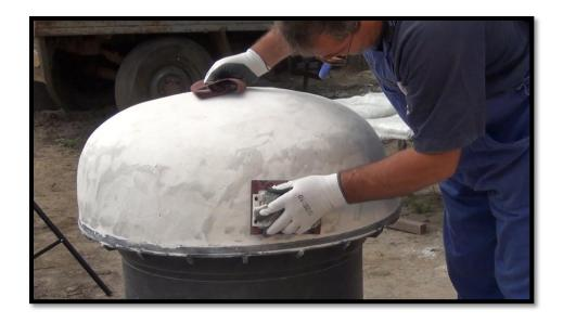
Before applying the fiberglass on top, I prepare the surface with floor wax so it won't stick to the plaster and it will be easier to get the hemisphere out of the mold.
