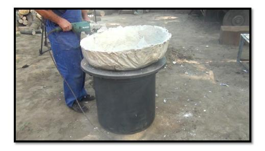
Now I will refine the surface to make sure that I will get a nice surface when laying the fiber glass on top.
