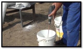
I begin placing one layer of plaster on the walls then add fiber glass mesh to make sure the mold won't crack when it hardens.
