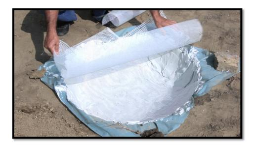
Don't worry if you are not getting a nice finish on the interior, the outside part of the mold is what we'll be using to lay the fiber glass on top.
