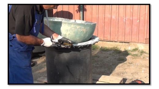
I insert some self-drilling screws to secure the fiberglass dome.
