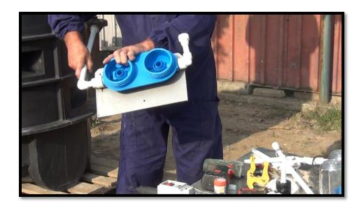
I am using screws to secure the filters battery to our piece of bond which will be attached to the biogas digester, in order to keep everything together.
