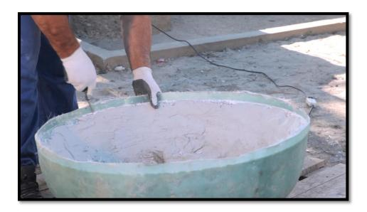
Hammering the fiberglass will release the plaster, making it easy to separate both pieces.
