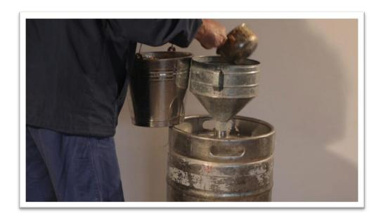
I will fill the second barrel with cold water, so the steam coming from the aluminum barrel is being transformed into liquid when it pass through the cold copper coil.
