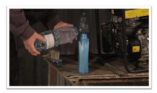
Now I am going to mix the regular gasoline with ethanol and start this generator.
