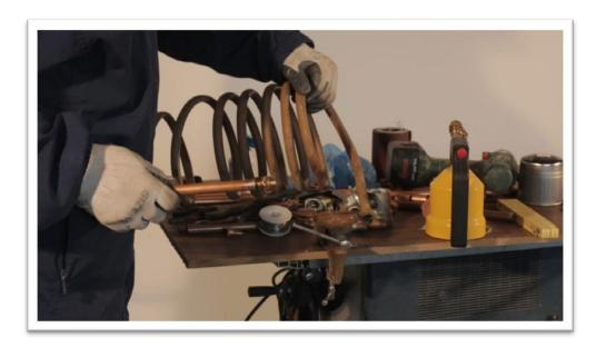
I am using pipe sealing string when connecting the pieces together.
