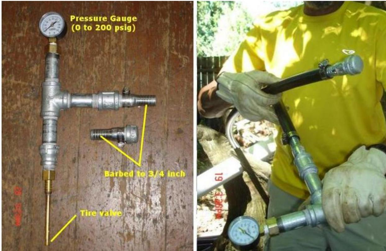
Left side shows the tester. Something to note is that I brazed the tire-fill stem on. It's important to remember to remove the valve core BEFORE you braze, and only reinstall it after everything cools down.
