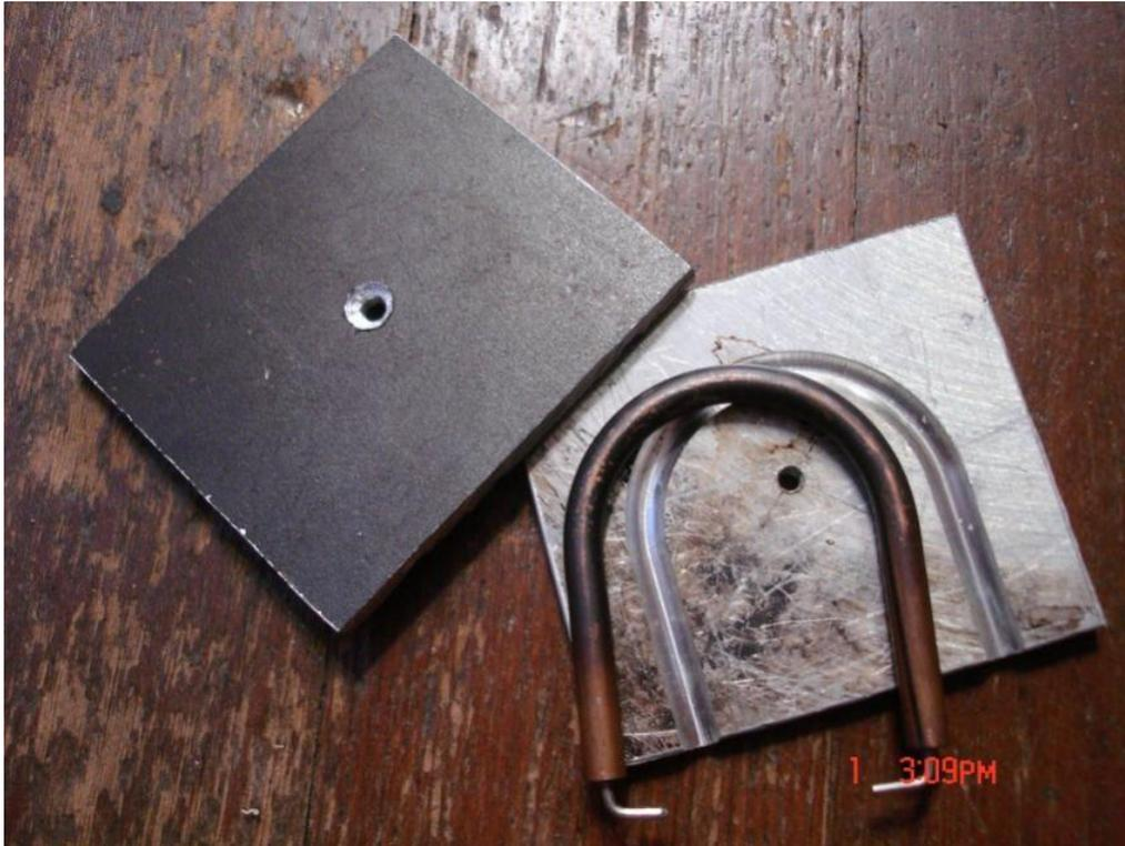
This shows the plates milled out to accommodate the heater element. I also milled a plate on my drill-press using a quarter inch drill-bit. It looked like hell but worked. Howard has a NC shop and did a perfect job in just a few minutes (shown). Not shown in this pic is a channel I drilled out to receive the temperature controller probe.
