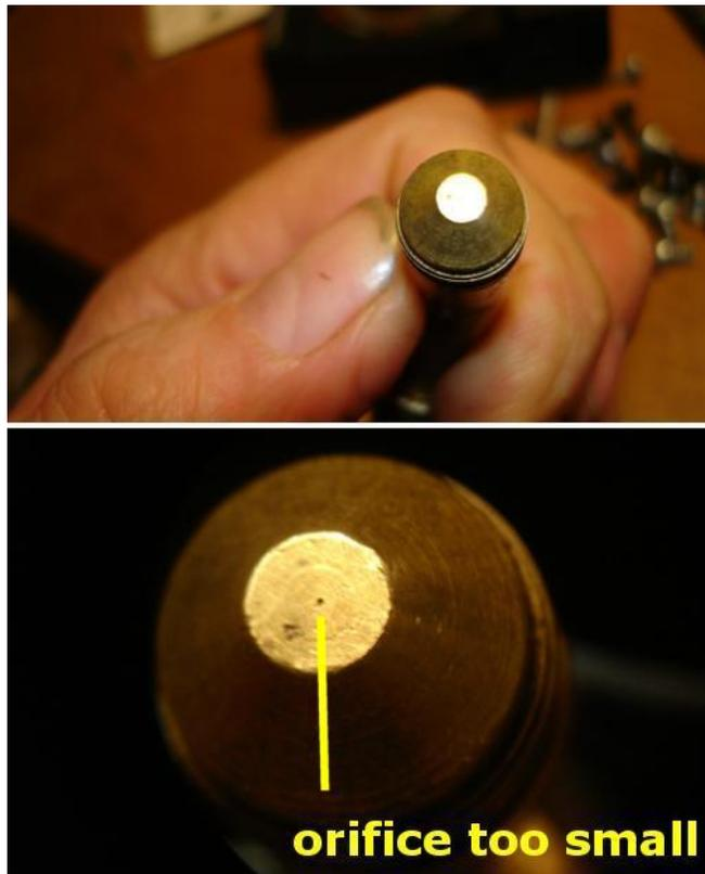
The orifice is a small hole at the end of the torch tube. It is so small you might not be able to even see it. As I recall, I got some pliers and just unscrewed the orifice brass part and threw it away. (It could also be drilled out)
