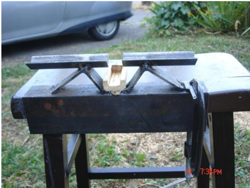
I did improve this jig from previous photos by using a wooden rest for the heater. this rest perfectly centered to heater on the pipe.
