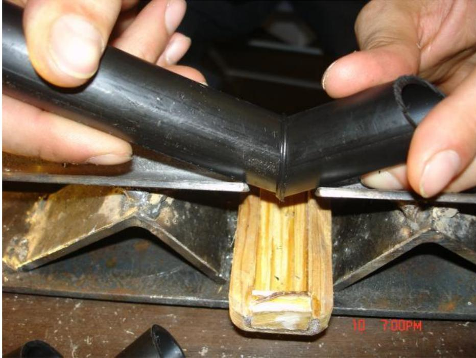
After using the jig in this manner, I realized that for small pipe, like 3/4 to 1 inch, hand joining is quite feasible, but having a jig of some kind to steady the pieces is very helpful. I also realized that a welded steel jig is not at all needed, and that a wooden or plastic jig would work also. In fact, even a tin can with the edges bent in like this would work just fine:
