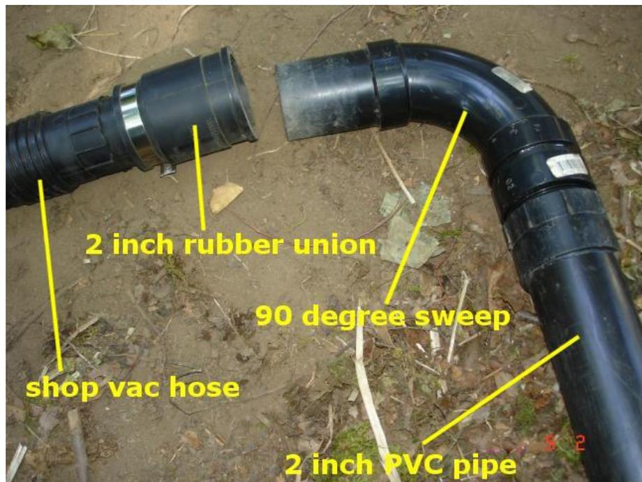
I use the hose clamp on the shop vac side, and use the rubber side loose on the PVC side. When the shop vac is running, the suction keeps it all together very well. The surprise benefit is that the 90 degree bend gives me a handle for rotating the pipe. And best of all, no more vacuum-hose kinks.
