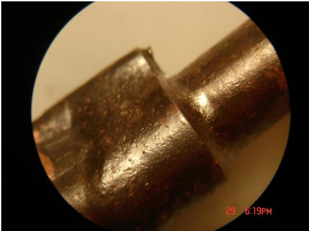
...but when I cut the joint out, all these black flakes of copper oxide fell out too. This will never work for refrigeration.
