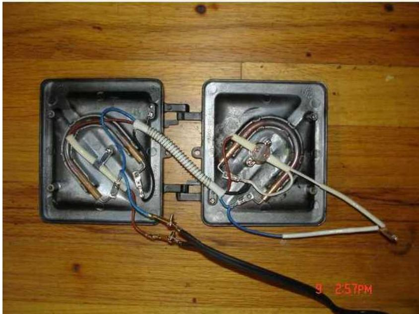
This device drew 600 watts, which I properly guessed ran 300 watts per side:
