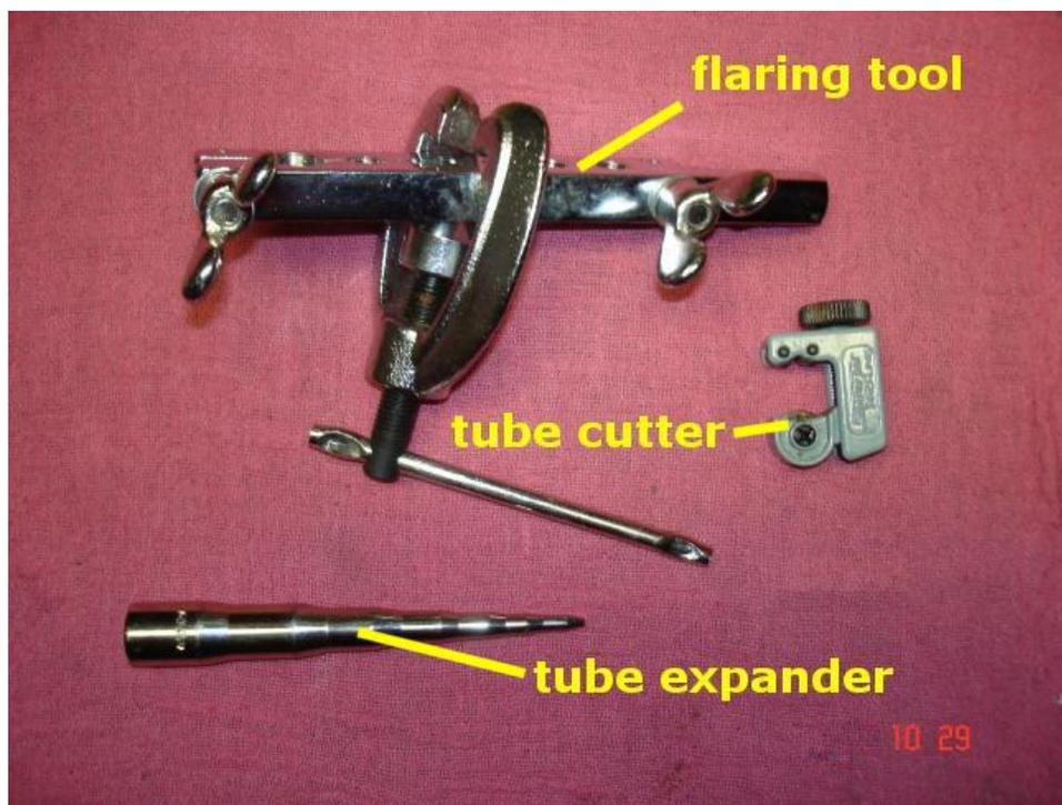
The flaring tool is usually used for making the flare for a flar fitting, but in this session, I'll be using it as a vice and as a heat sink.
