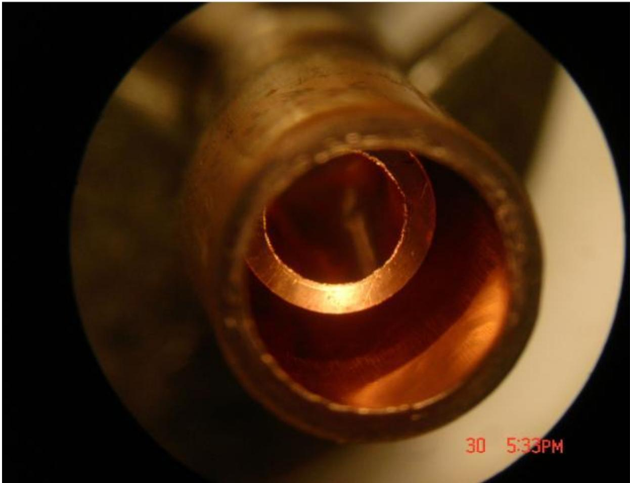
Bottom photo tells why... This is a microscope shot down the barrel of the tube I just brazed. The cut was made about 3/4 inch from the brazed joint and about 5 minutes earlier, it was glowing cherry red. As you can see, there is no copper oxide, not even any discoloration.
