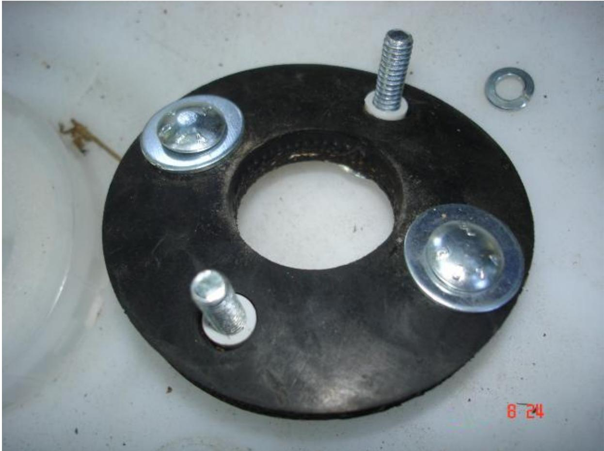
So I tried a Ford/GM steering doughnut replacement part, set up the way it was designed and it worked just fine for about three glorious, high-stress minutes before failing.
