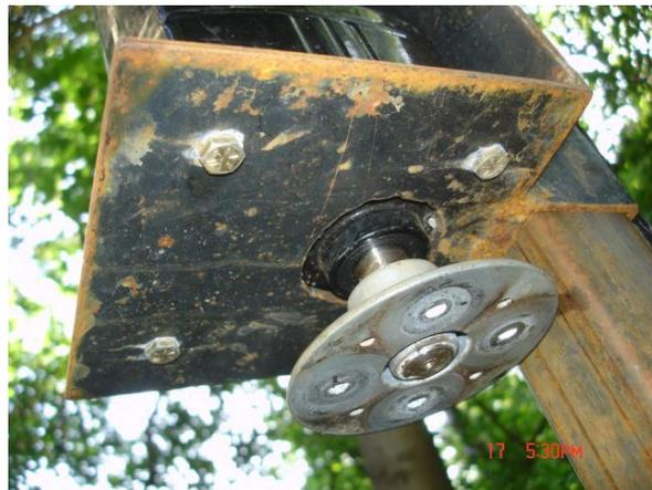
Here are the vibration dampers I use to tie the two flanges together. I use nyloc nuts to prevent them from backing off during use. Works great.
