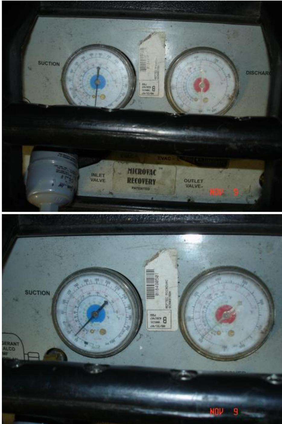
Then the valve knobs are turned to the "Evacuation" position, and the needle valve on our storage bottle is opened. You will see deflection of the gauges as the refrigerant is pumped from the AC unit, through the Microvac, and into the storage bottle, as shown in the lower photo. The unit is run until the
