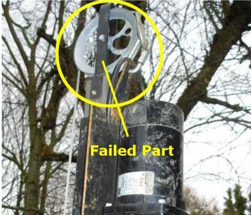
I was trying to extract an auger from the hole #16 and the forces generated by the 2000 pound winch easily deformed it.
