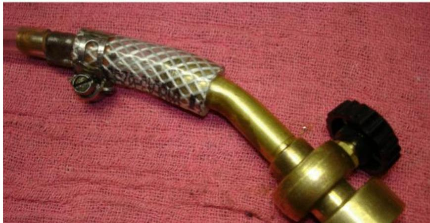
First I unscrewed the flame tip from the propane torch, which was worthless for brazing anyway.
