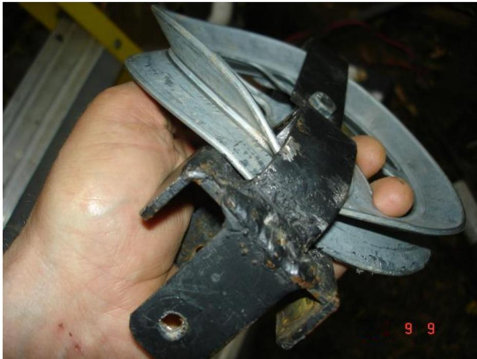
I wasn't terribly surprised as the pulley was actually made for reeling in clothes line. I had estimated correctly that it was a good match for the manual winch, but the power winch was just too much for the
