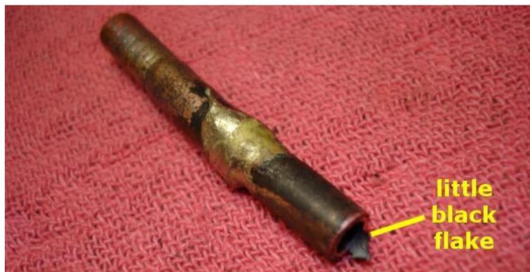
So all the lovely heat of the MAPP gas has caused the copper in the tube to combine with oxygen and make this flake of copper oxide. This is **VERY BAD** for refrigeration, because the refrigeration circuit relies on liquid refrigerant passing through a capillary tube or a tiny orifice to regulate the flow rate. Just one flake of copper oxide could ruin the whole thing.
