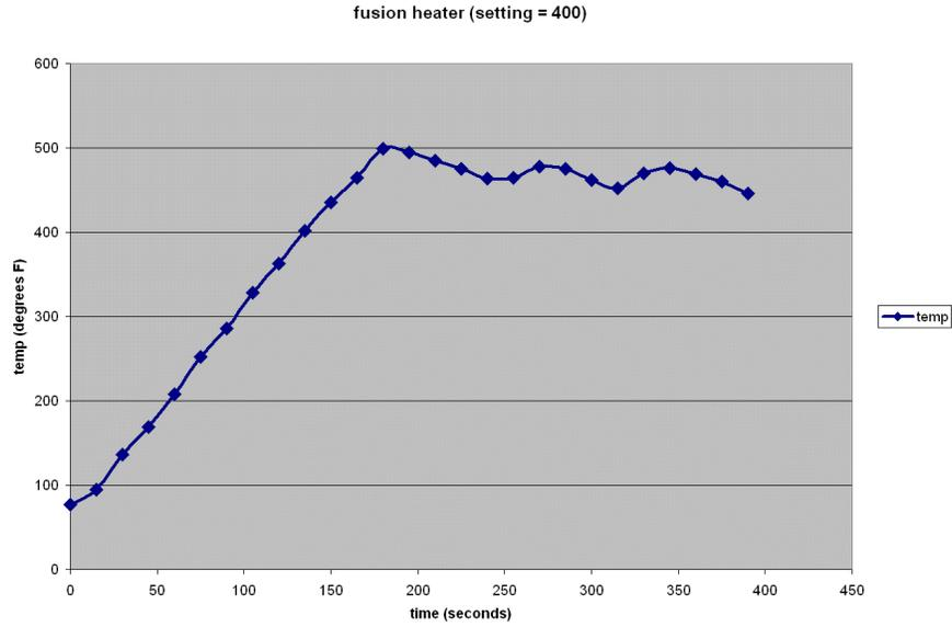
This is a graph of the unit heating up when the dial is set to "400".
