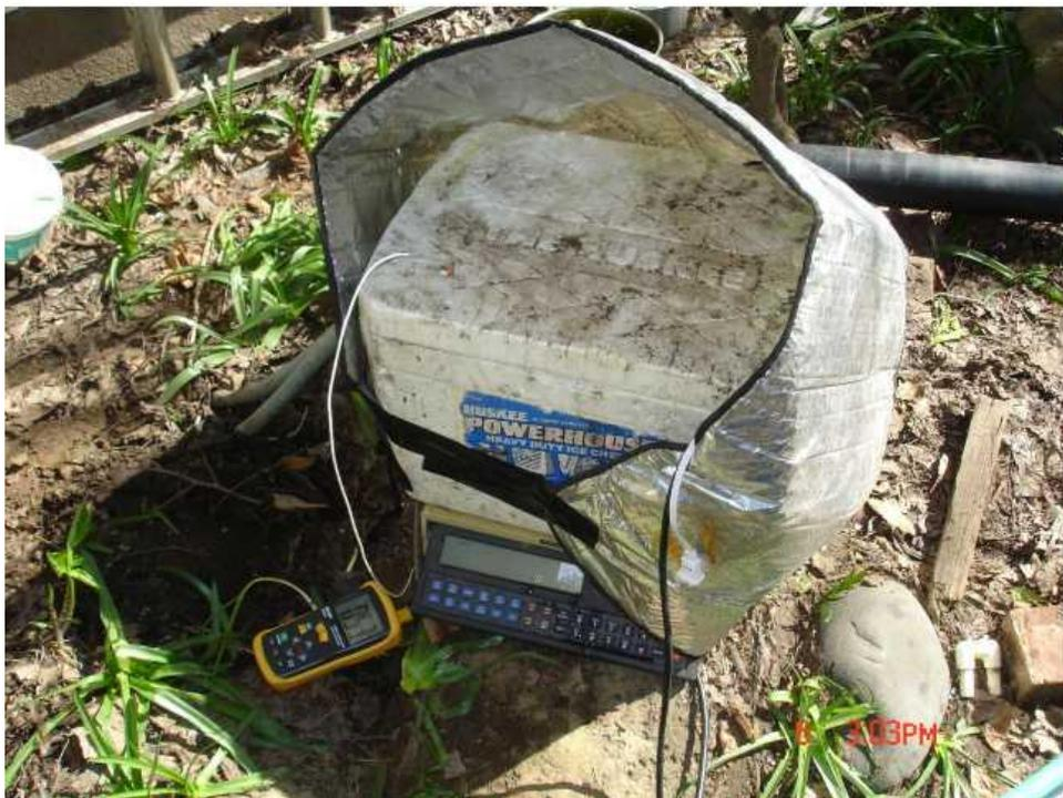
this shows the set-up in the cooler box. I initially thought that it would be a good idea to put the coffee cup warmer inside of something so it wouldn't melt the foam box. I nixed this idea, and suspended the heater from the hose with a bread wrapper twist-tie.
