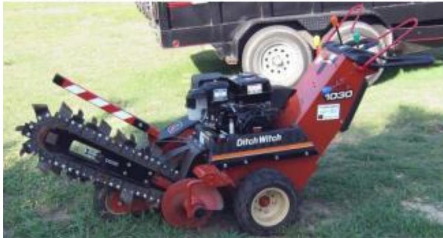
We selected a Ditch Witch which was probably second choice, but it did have the advantage of being 'maneuverable'. It turns out that this type of machine has no real steering, it just goes backwards in a generally straight line and digs as it goes. Changing direction is not easy and consists of grabbing this horribly heavy machine and using all of your strength and moving it a few degrees, then repeat until properly positioned.
