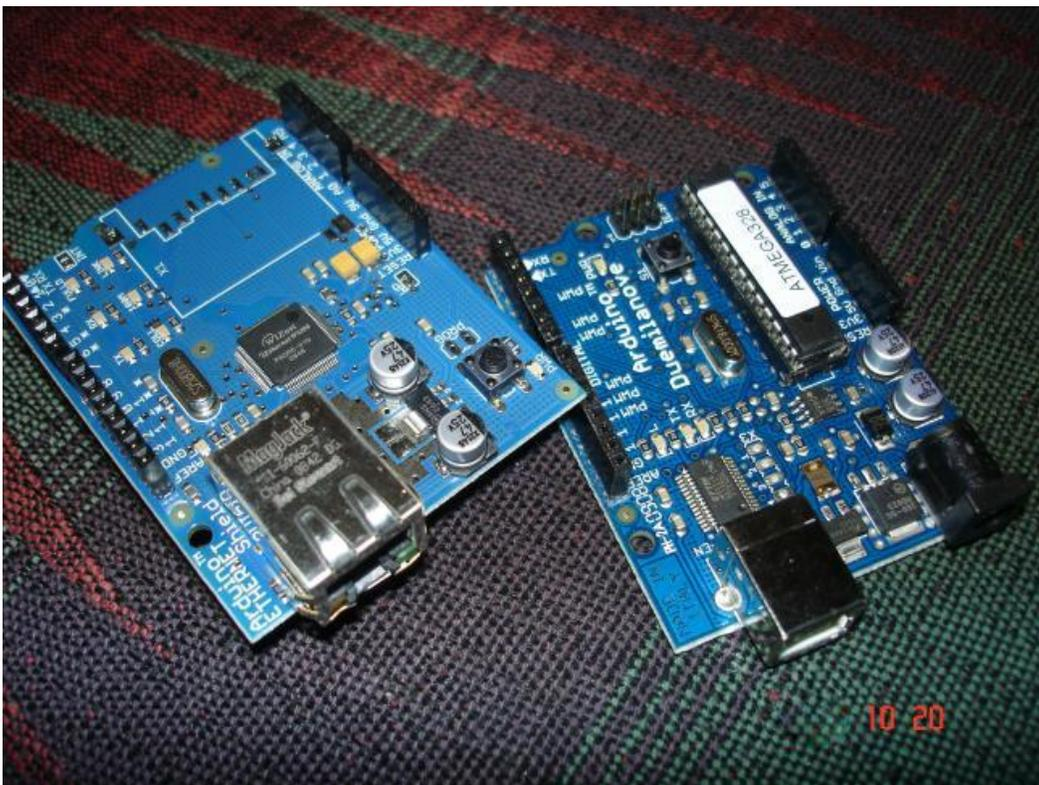
I got both of these boards from Spark Fun. The one on the left is the Ethernet Shield and the one on the right is the Arduino board.
