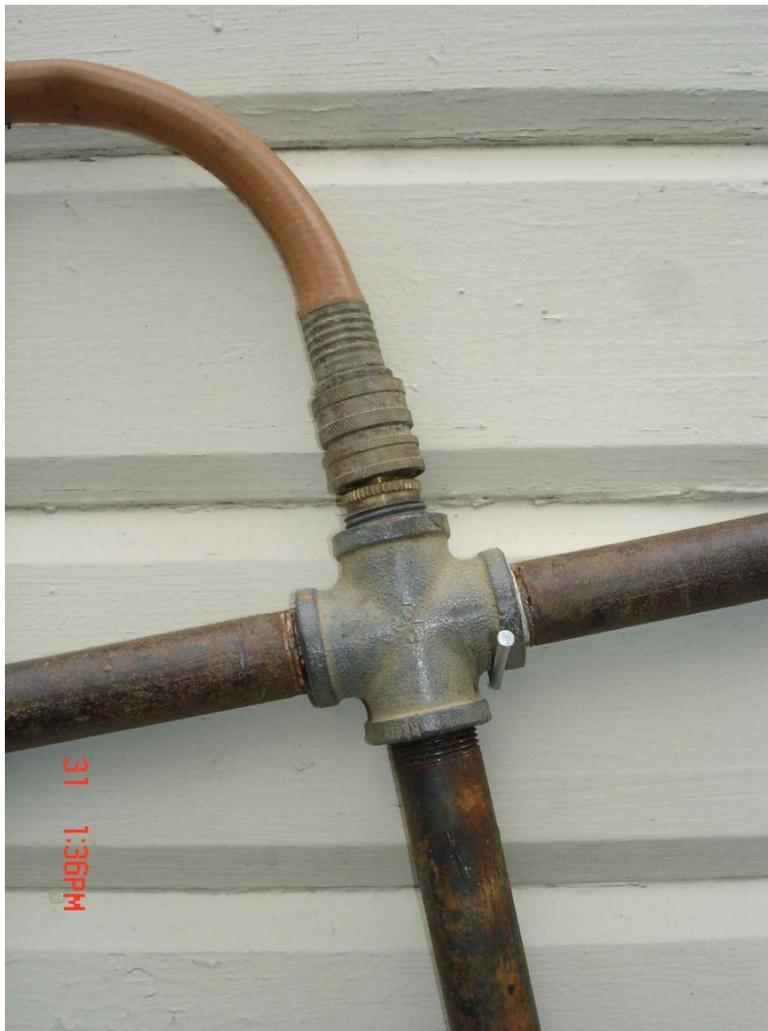
This is a detail of the swivel end of the auger. The swivel adapter is not exactly the same as 3/4 pipe thread, but by loading lots of teflon tape onto the threads, I got a satisfactory seal.
