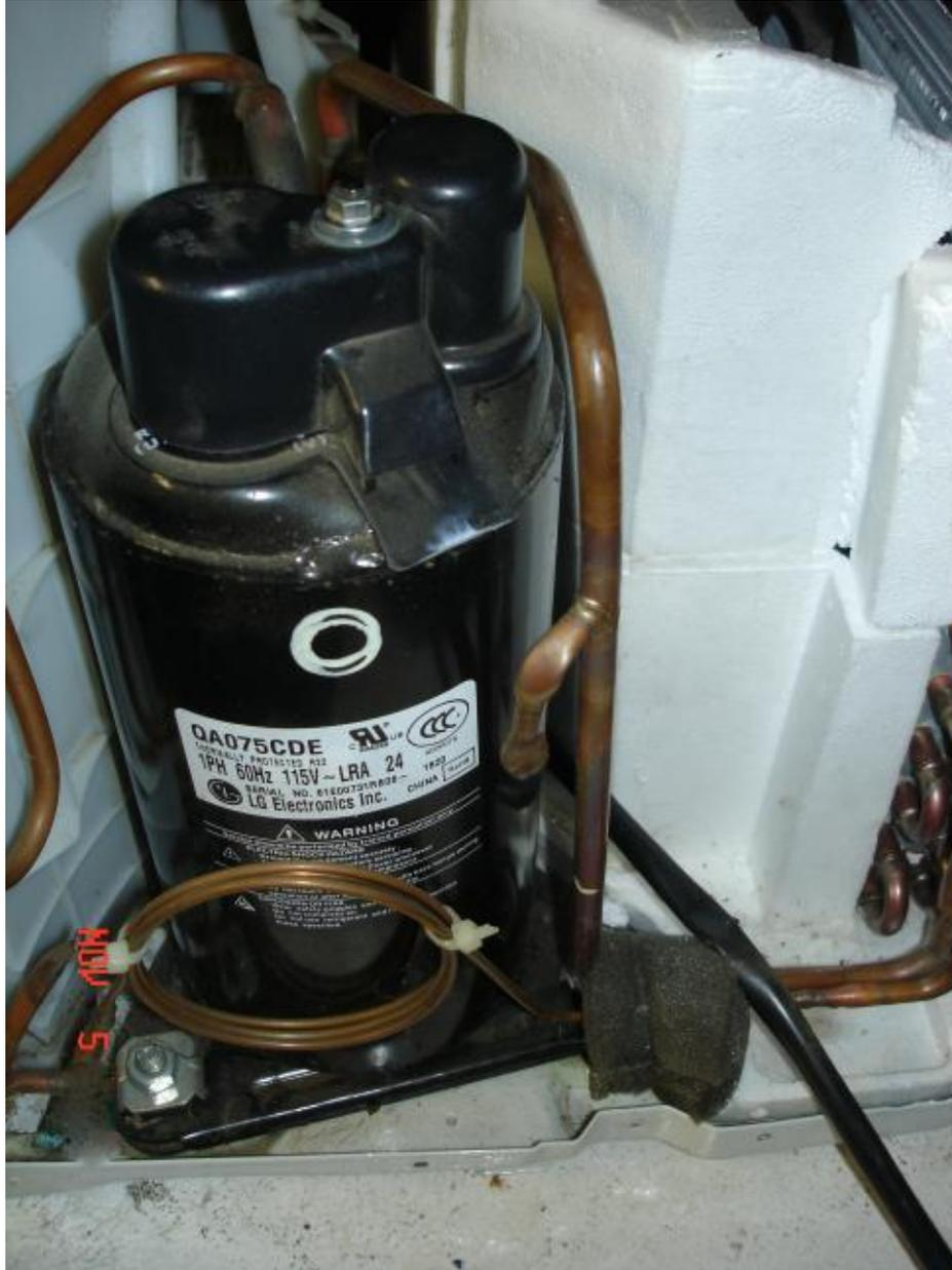
Notice the small coil of very thin tubing that is near the bottom of the compressor...
