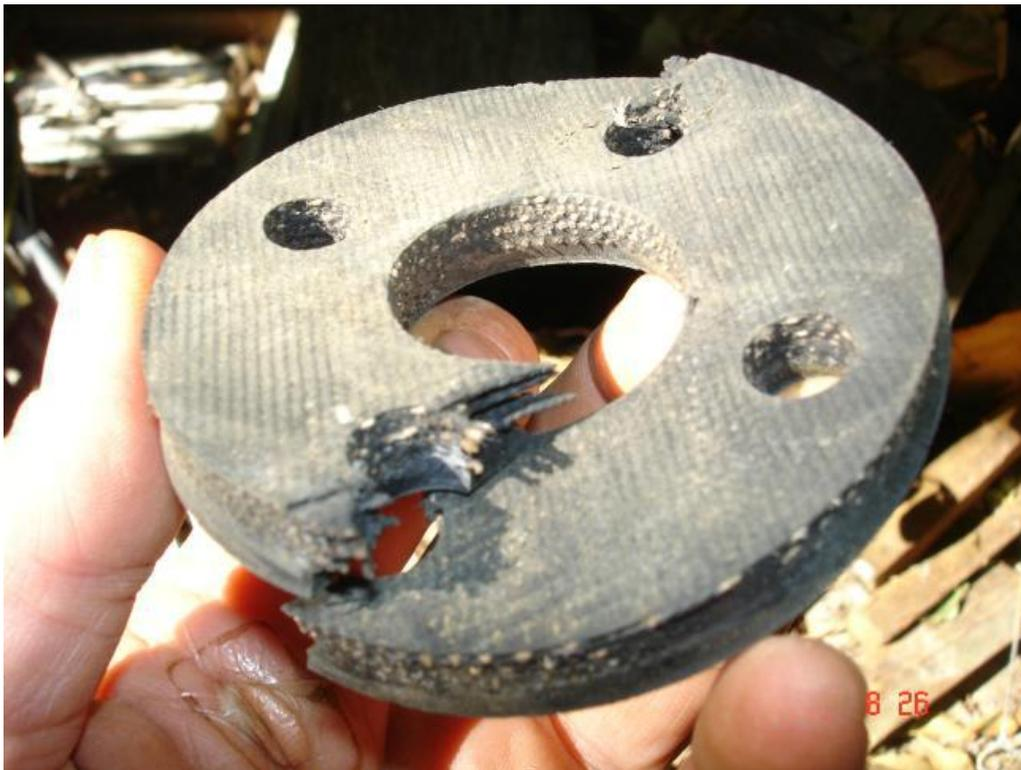
So my solution was to use stainless bolts to bolt straight through the doughnut and add some rubber washers atop the flanges capped with big washers, and adjust the nyloc-nuts to 'barely snug'. Under off-
