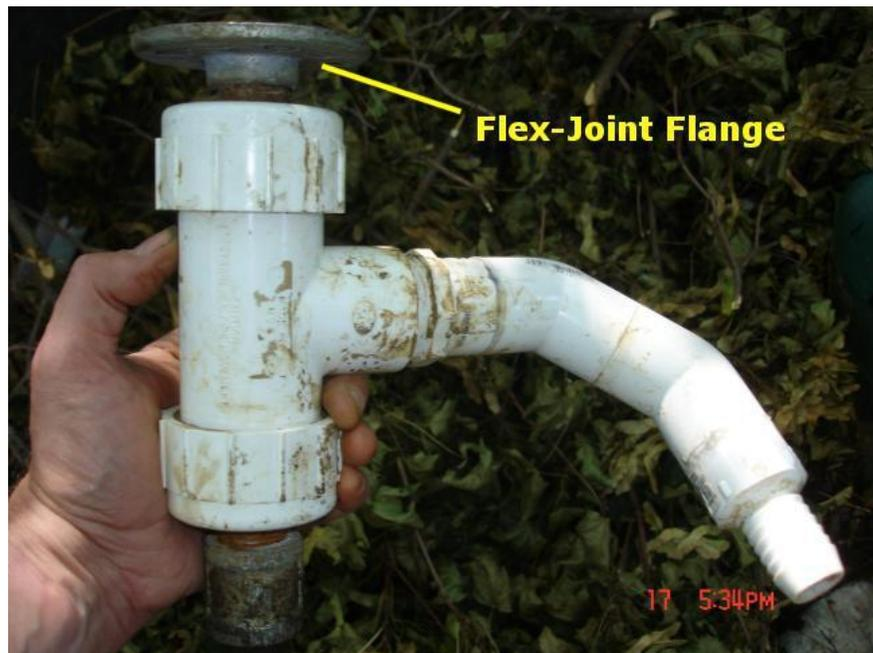
And here is the repaired and complete flex-joint, ready for more drilling.
