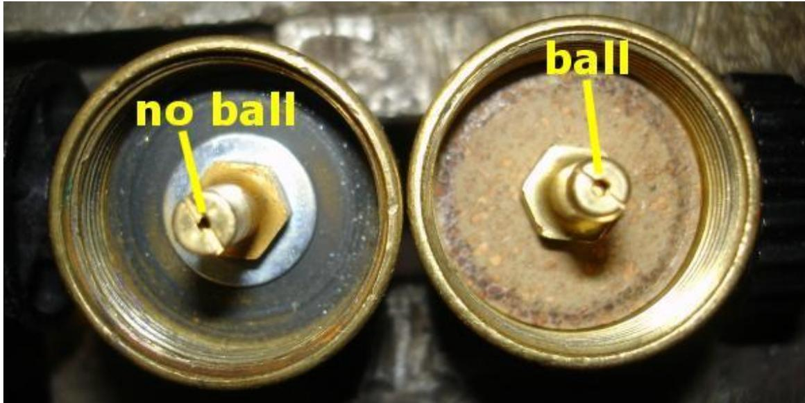
I just unscrewed the stem and removed the ball, then put the stem back on, minus the ball.
