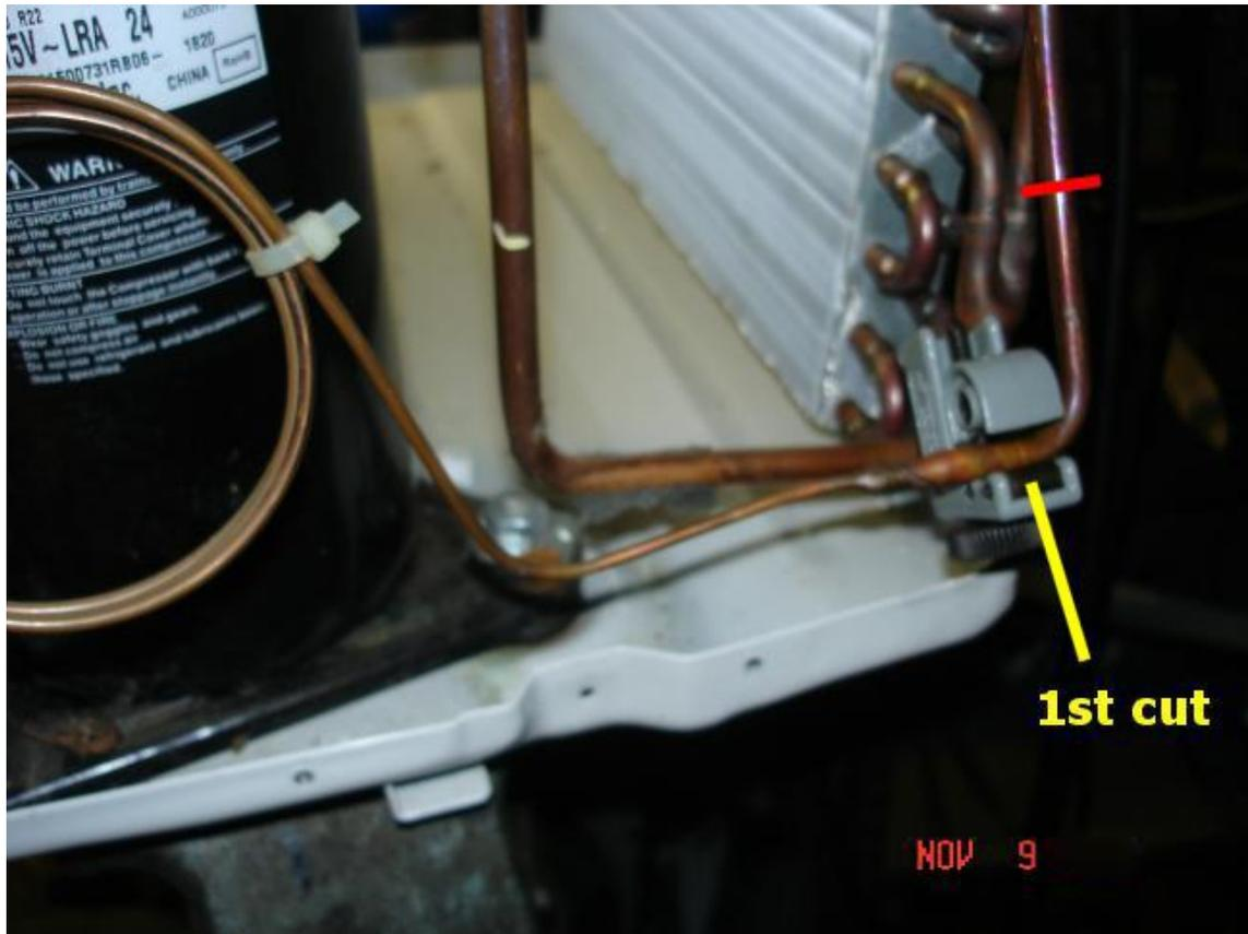
I have made a red mark on the photo to indicate another good place where the cut could have been made...
