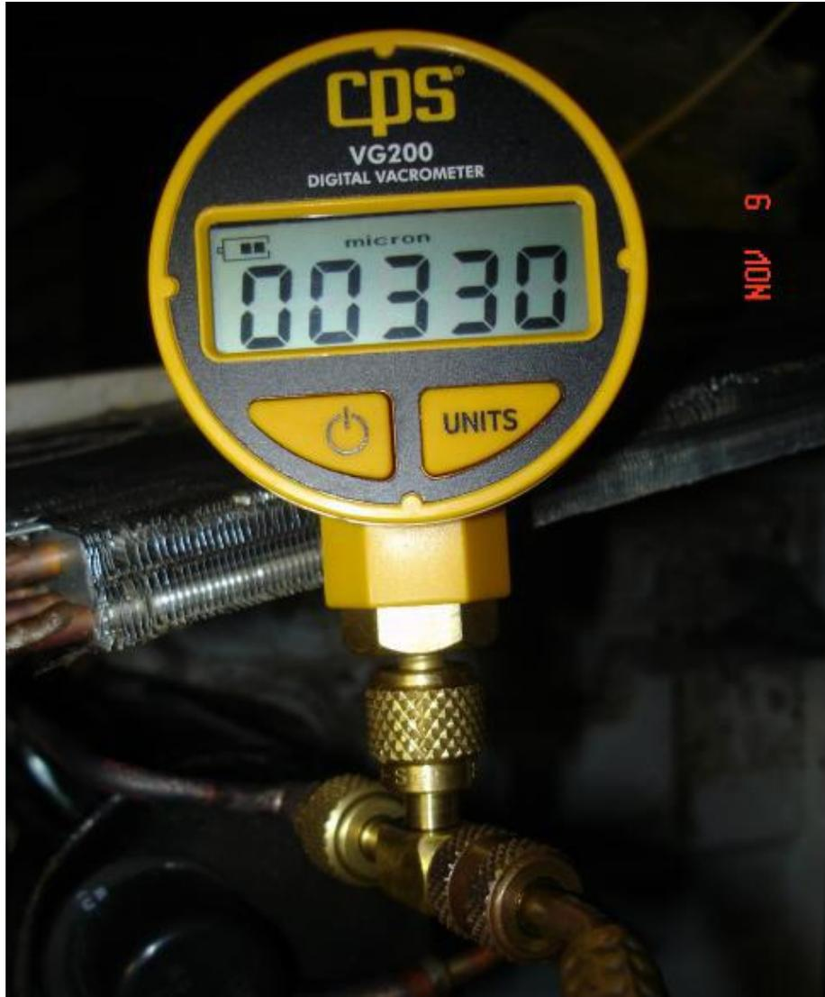
Before I put in the core, I pulled a vacuum with a micron gauge attached, and quickly hit 330 microns, so I took that to be 'no leak'.
