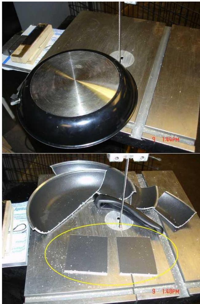
This will give me non-stick surfaces for fusing the poly pipe.
