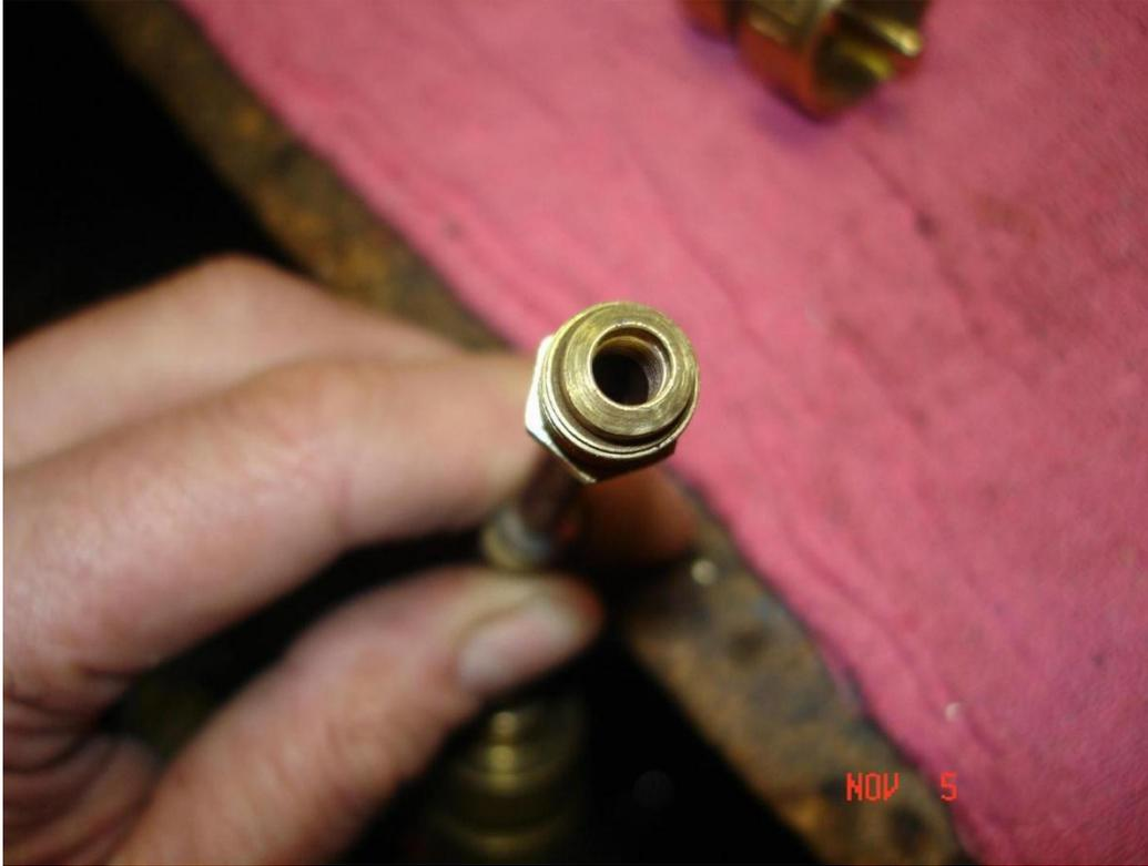
I didn't put the Schrader core back into the valve, because with the needle valve of the torch, there's not much need.
