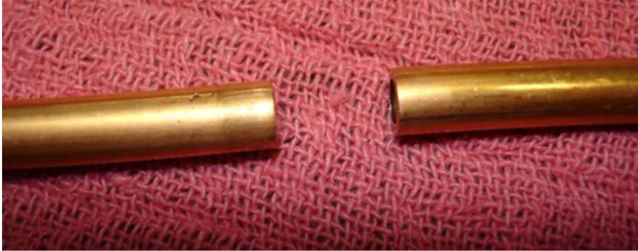
Since refrigeration is subjected to vibration, a butt joint will not do, so the trick is to expand one piece of tube so that the other tube will fit inside.
