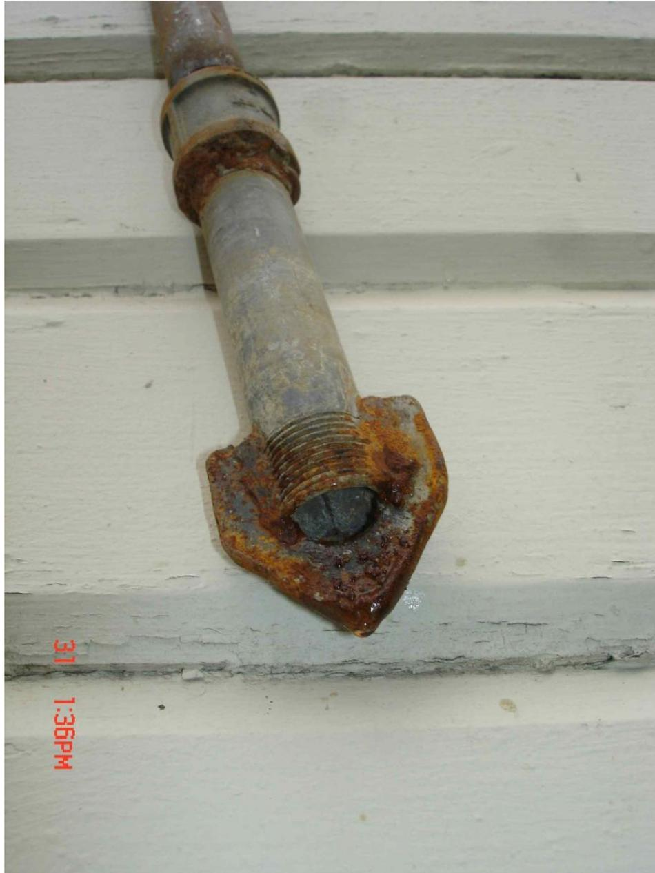
This is a detail of the business end of the auger. The water gushes through the pipe and flushes out the drill-cuttings. I have come to understand that the water is definitely part of the tool. It contributes more to the advancement of the drill than any effort on my part.
