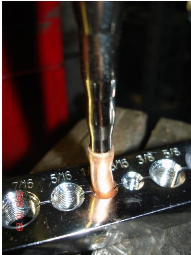
Here I'm using the flaring tool as a vice and I'm tapping the tubing expander with a hammer to stretch the tube to the right size. I'm actually going two steps bigger, so the tubing got a bit deformed, but it ends up being a sound joint.
