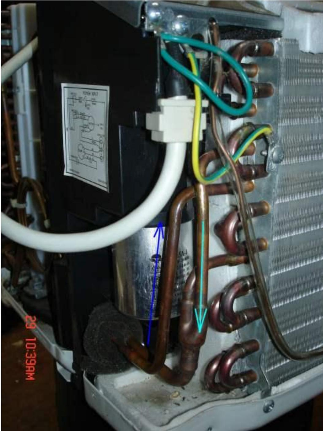
I have drawn the flow arrow to the condenser in BLUE to indicate that it is really cold, and the flow arrow from the condenser in LIGHT BLUE to indicate that some of the cold has been lost, actually heat has been gained.
