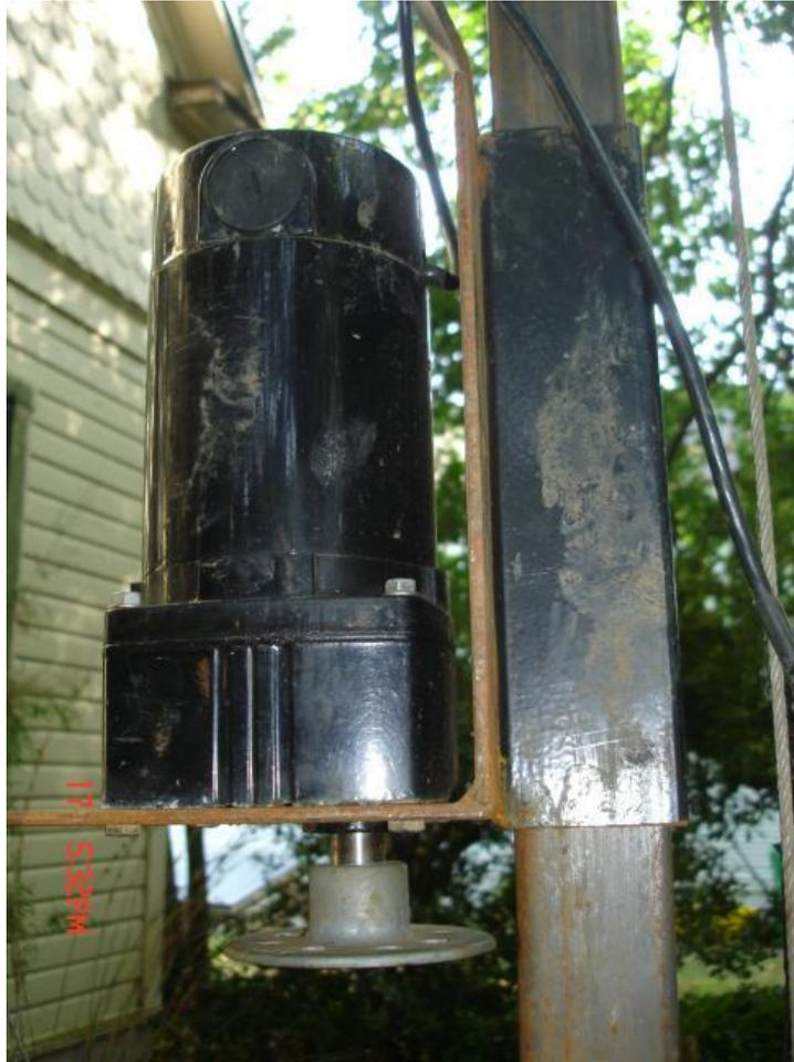
I welded the motor bracket out of 3/16 steel. It could use some reinforcement at the corner.
