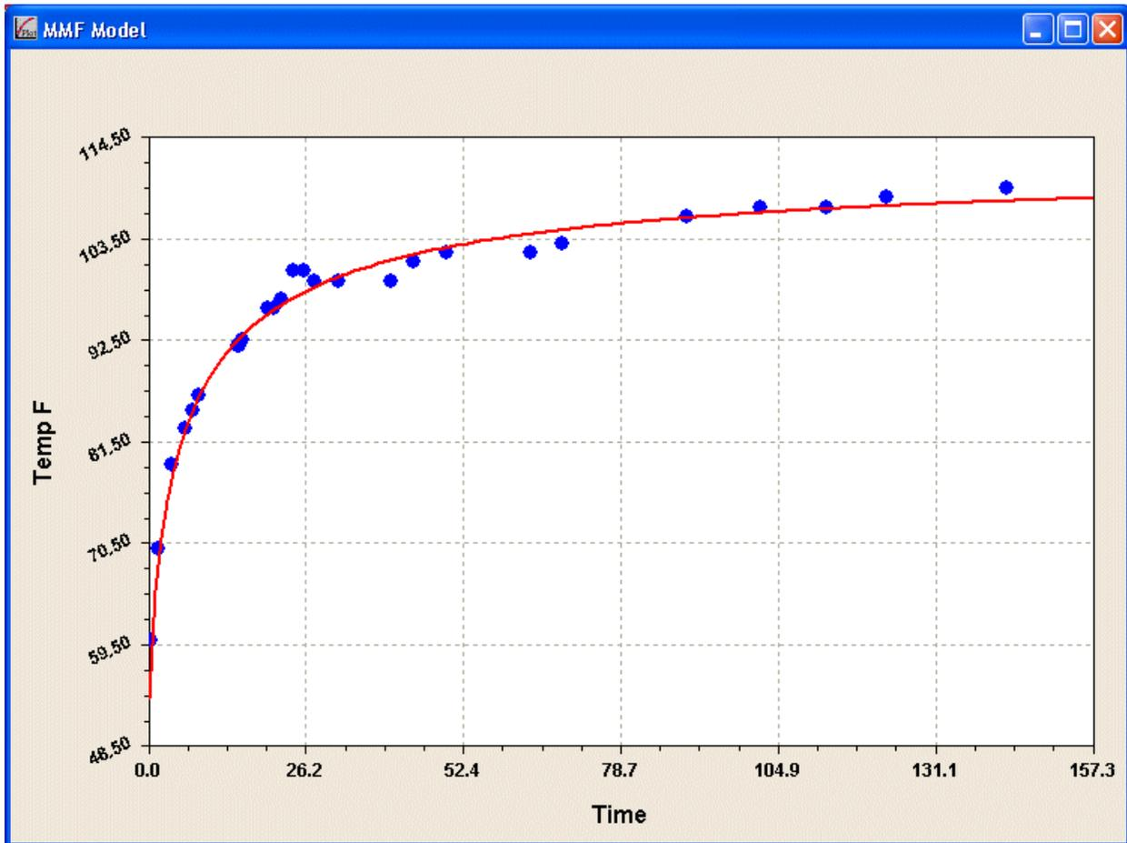
From CurveFit, it's even possible to get the equation of the curve that is the best fit and to project the curve forward in time. I was interesting to predict what the temperature would be at a particular time and to check the results as they came in.
