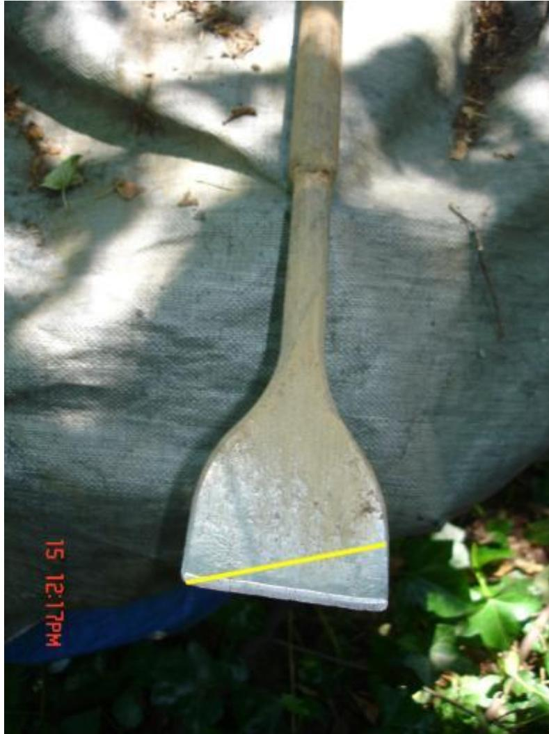
...this tool would have been improved by grinding the chisel at an angle indicated by the yellow line. The root-hacker tool was also useful to loosen the dirt at the bottom of the hole as we went deeper.
