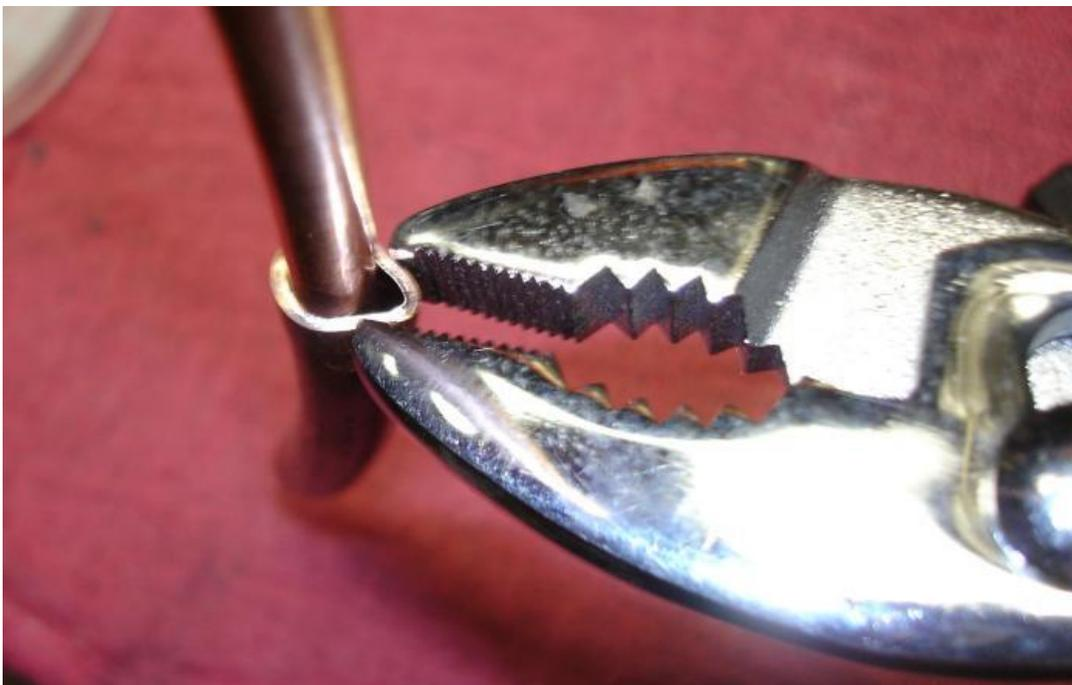
We put the smaller tube into the bigger tube and grab the edge of the big tube with a pair of pliers, and pinch...
