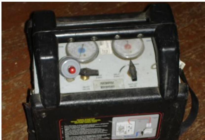
Basically, they are both turned to the "Self Evac" position and the unit is run until a full vacuum is pulled, as shown in the top photo below.
