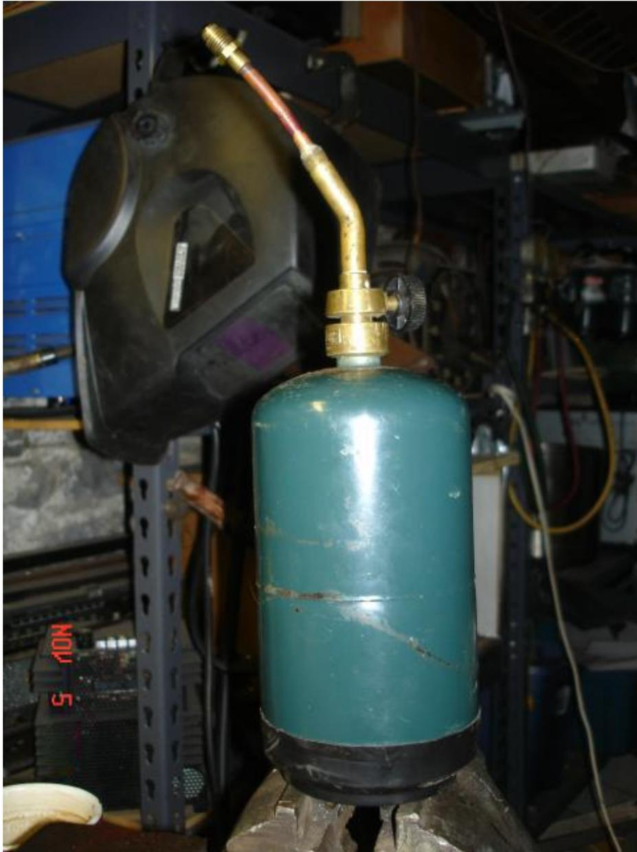
The beauty of using propane bottles is that each one has it's own ball-valve built into the bottle to prevent gas from escaping. When you remove the torch from the bottle, you can hear the ball-valve
