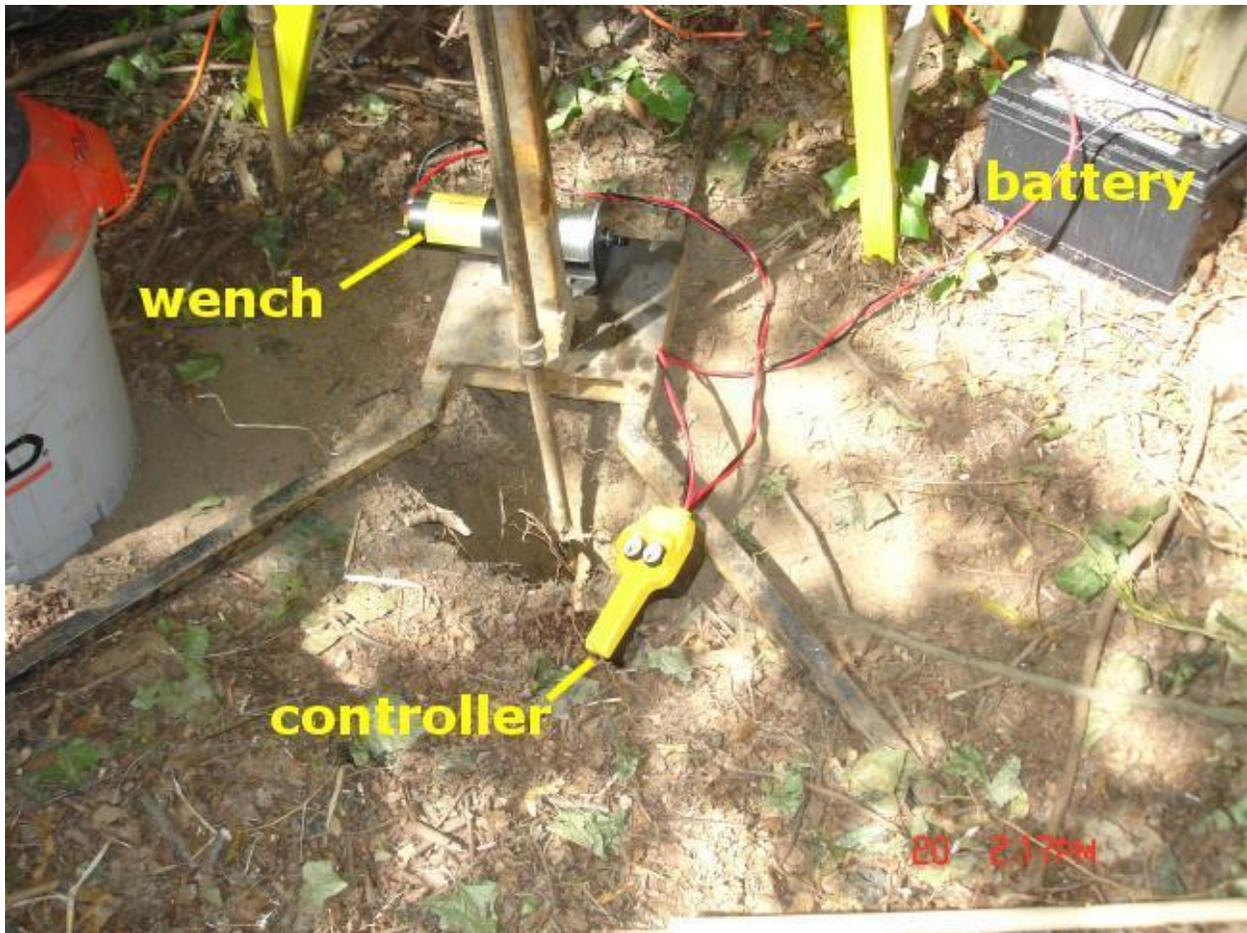
After I have managed to get through the layer of clay at 4 feet, the soil composition becomes a mixture of brown sand and clay, with the percentage of sand increasing as I go deeper. Here the electric auger works just fine, and has saved me loads of hard manual work.
