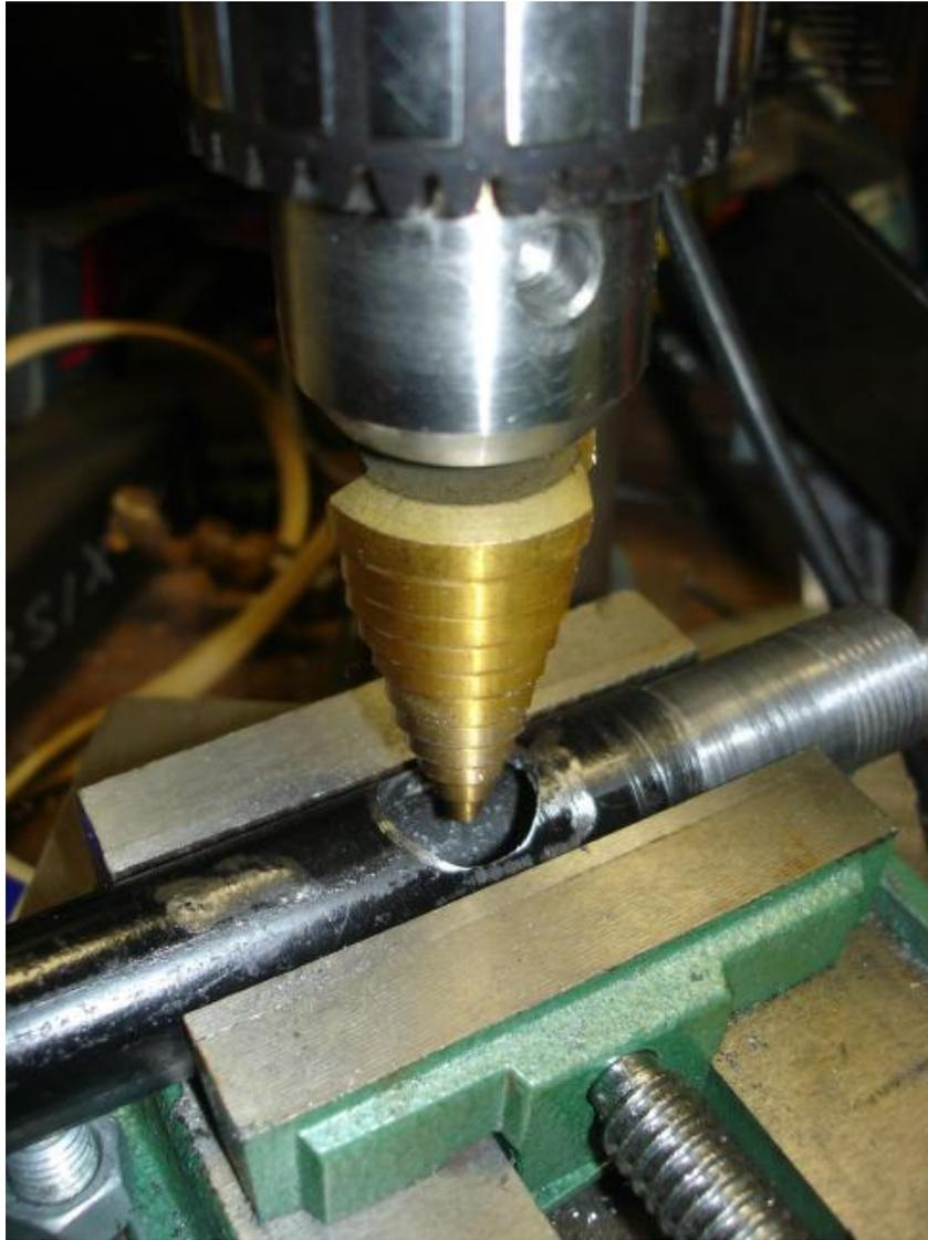
...so you'll want to stagger the holes and both holes should have a combined area a bit bigger than the ID of your drill pipe.
